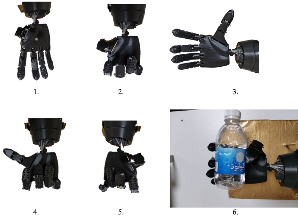
Fig. 7 The prosthetic hand movements: (1) Hand shake, (2) Fingers closed, (3) Fingers open, (4) OK gesture, (5) Half open, and (6) Grabbing an object.
