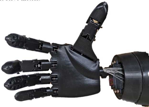
Fig. 5 The 3D printed prosthetic hand.
